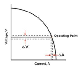
Relationship between the voltage and current for different process in CC type power source is as under
