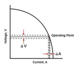
Relationship between the voltage and current for different process in CC type power source is as under
