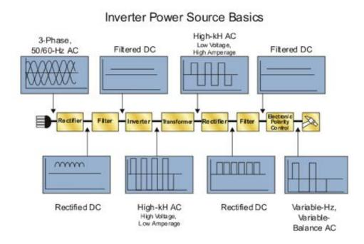
Different types of power sources are available for welding and most commonly used are as under
