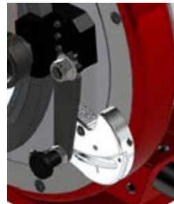
Outer profile guide system: to account for tube "out of round"
