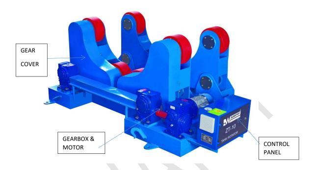
Once the Rotators are received at your end inspect for proper condition of the equipment then choose the proper place for Rotator installation.
