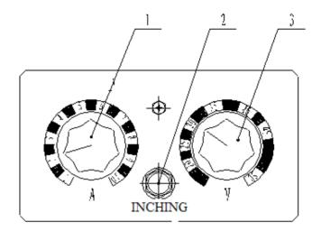
Fig. 6: Panel of controller
