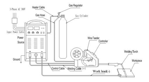
Fig.1: Wire diagram of IN MIG-I series welders
